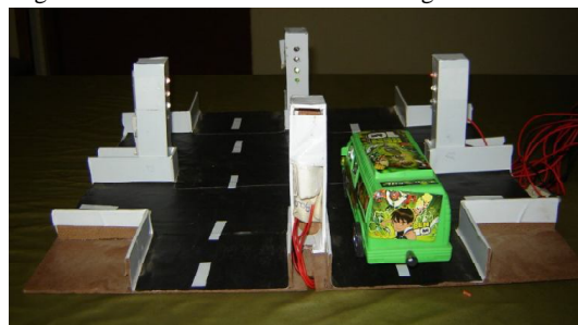
Figure 4. change of lights from red to green on siren detection
