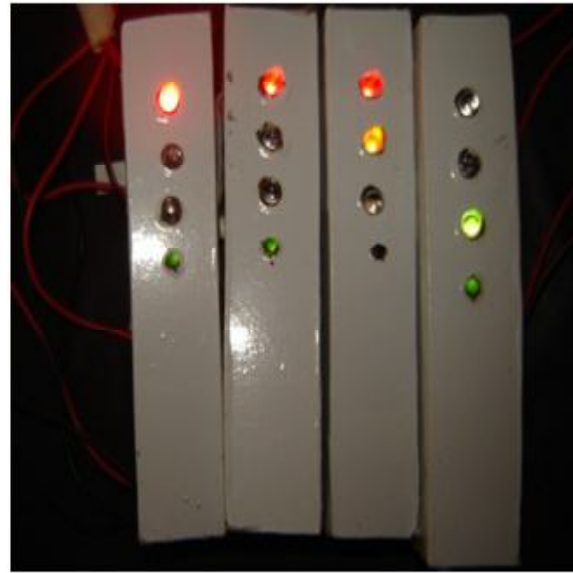
Figure 6. Lighting sequence of the traffic light after implementation
